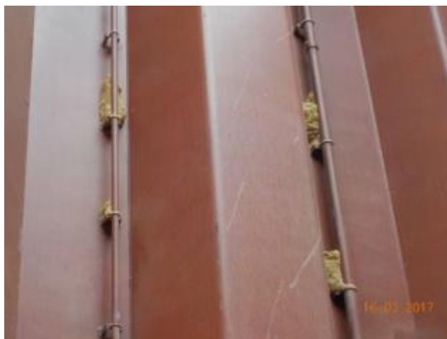
CARGO STUCK BEHIND PIPELINES
